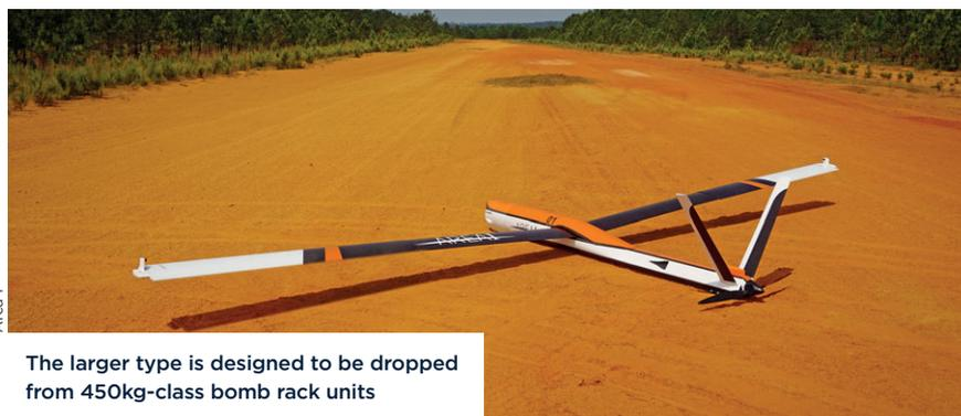
The larger type is designed to be dropped from 450kg-class bomb rack units
