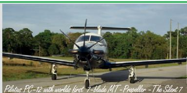
*Pediatric PC-12 with world's first 7-blade MT-Propeller - The Silent 7*
