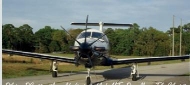
Pilatus PC-12 with world's first 7-blade MT-Propeller - The Silent 7
