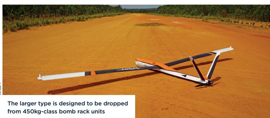
The larger type is designed to be dropped from 450kg-class bomb rack units
