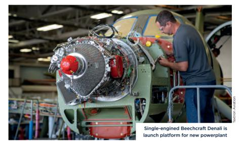
Tests have shown the Catalyst to be up to 16-17% more efficient than competing engines, one to two percentage points more than GE had anticipated, and with more power at high altitudes than predicted; performance gains that Corkery says are "not trivial".
