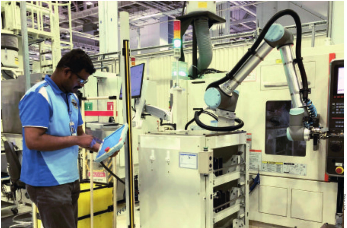
Pratt & Whitney component unit has improved quality control by implementing robotic inspections, engraving and machining loading
