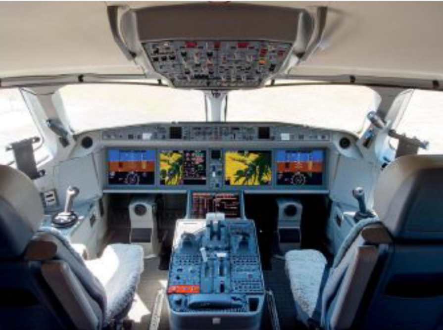
Design took advantage of sidesticks, fly-by-wire technology and advanced construction
