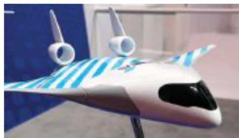
Airbus has been testing model of flying-wing design
