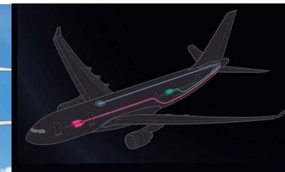
the APU will be replaced by a hydrogen fuel cell system, feeding a power distribution network.
