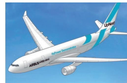
HyPower will have forward compressors and aft hydrogen tanks, with fuel cells in the tail cone
