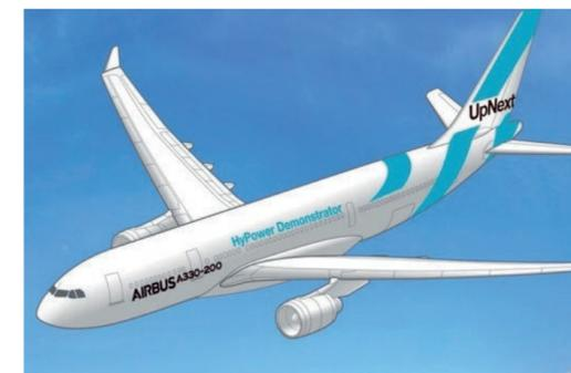
HyPower will have forward compressors and aft hydrogen tanks, with fuel cells in the tail cone
