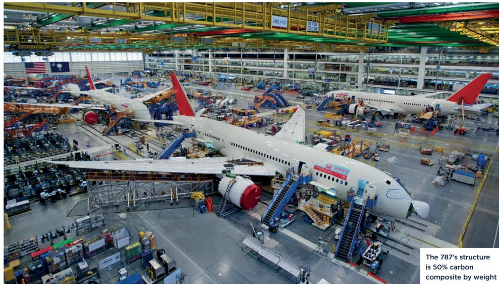
The 787's structure is 50% carbon composite by weight
