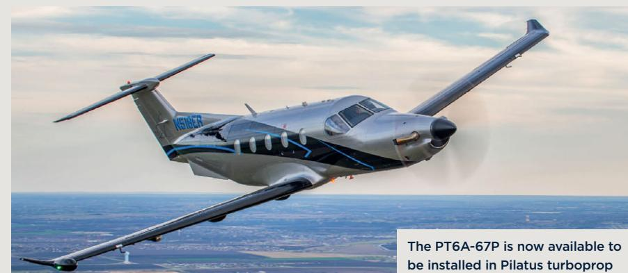
cruising altitudes. Where the stock -67B starts losing power at 13,000ft, the XP67P can maintain full power to 23,000ft.
