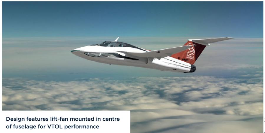
Design features lift-fan mounted in centre of fuselage for VTOL performance
