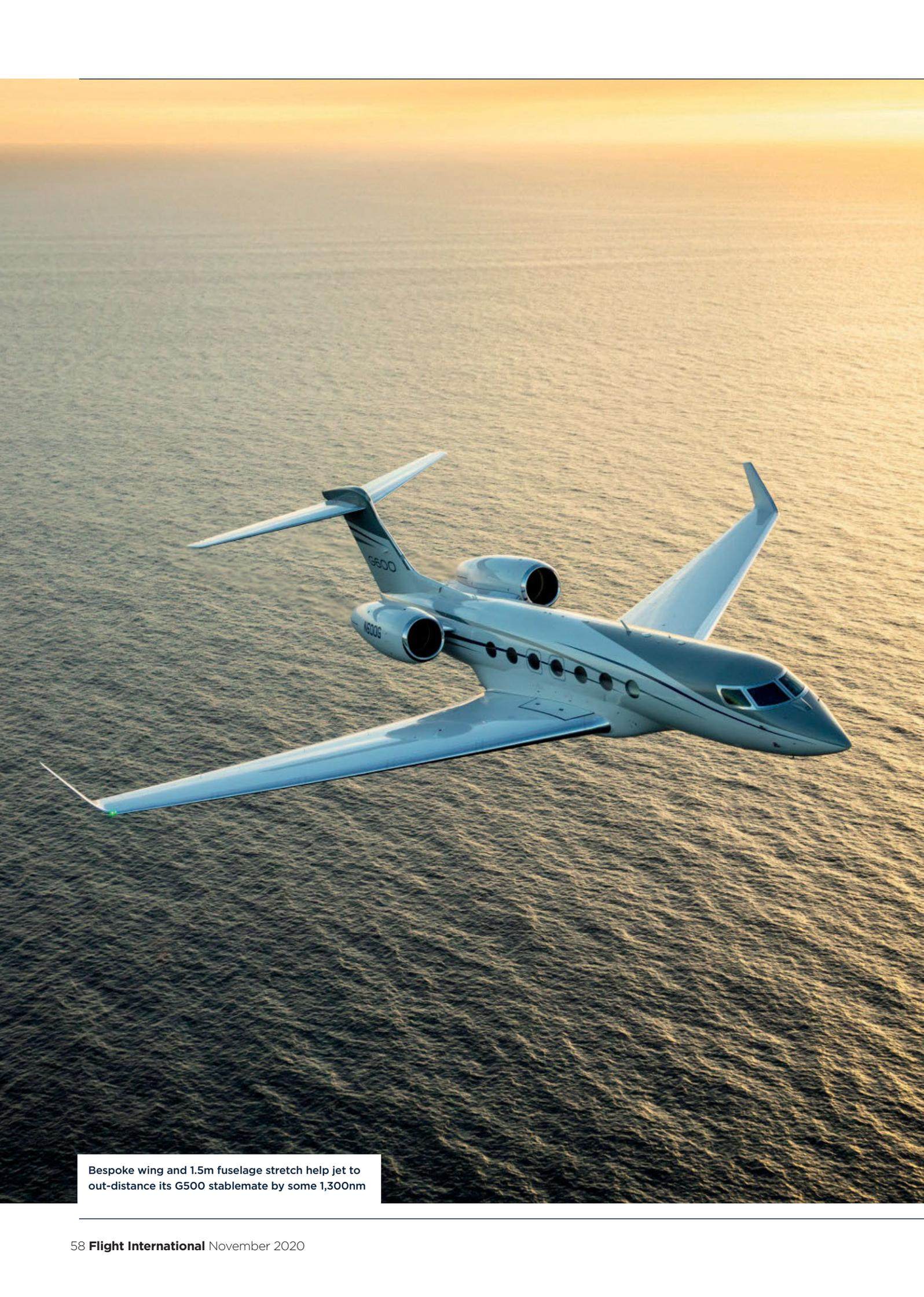
Bespoke wing and 1.5m fuselage stretch help jet to out-distance its G500 stablemate by some 1,300nm
