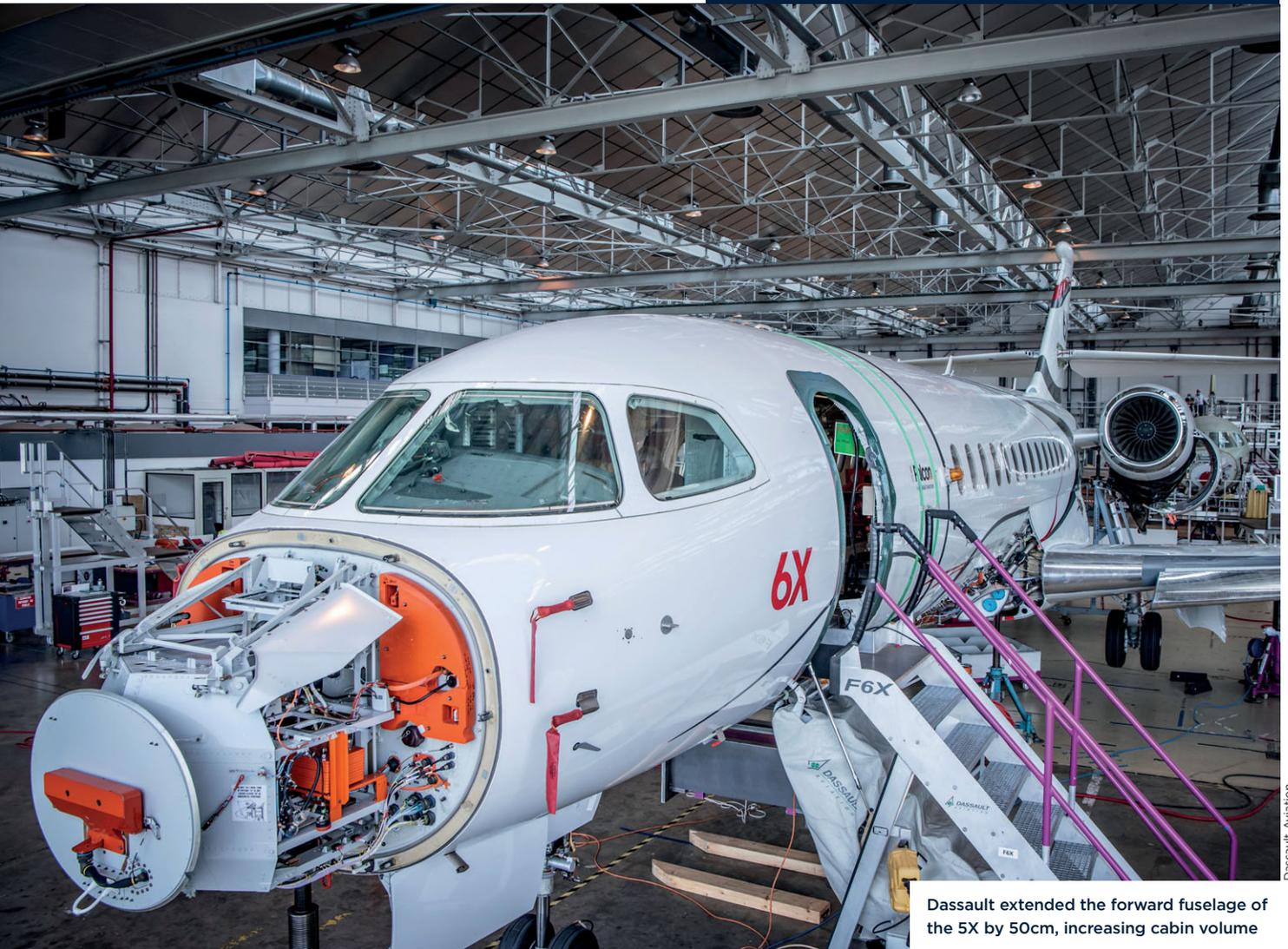
Dassault extended the forward fuselage of the 5X by 50cm, increasing cabin volume
