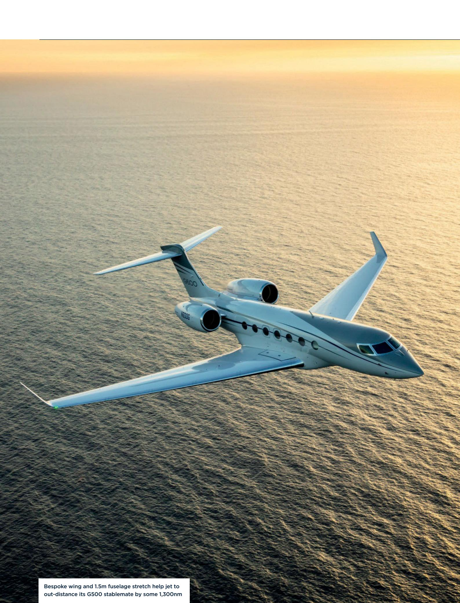
Bespoke wing and 1.5m fuselage stretch help jet to out-distance its G500 stablemate by some 1,300nm
