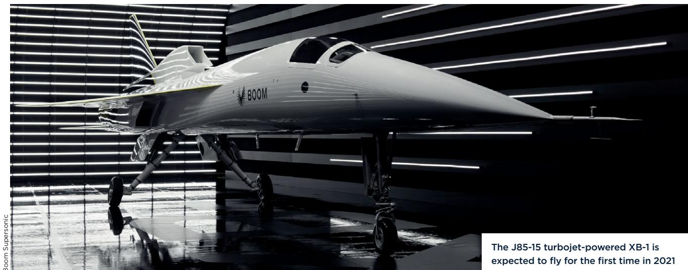
The J85-15 turbojet-powered XB-1 is expected to fly for the first time in 2021
