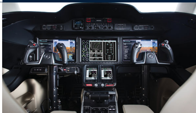
Cockpit features a Garmin G3000-based avionics system and has an uncluttered feel
