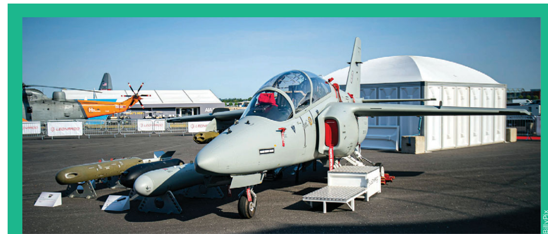
Attractions on show at Leonardo's outside exhibit area include a first glimpse of its M-345A jet trainer in an armed configuration. Currently flown by the Italian air force as the T-345A, the single-engined jet can be equipped with weapons including unguided rockets, bombs, gun pods and air-to-air missiles.
