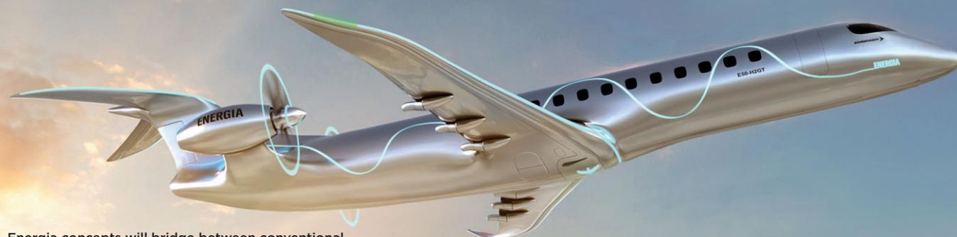
Embraer Energia concepts will bridge between conventional turboprop and hydrogen-powered variant
