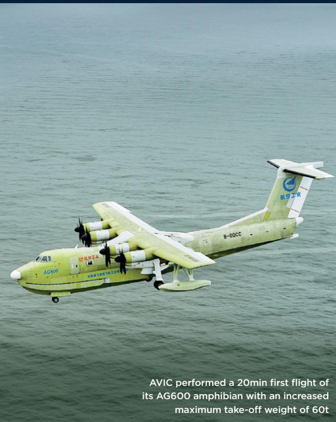
AVIC performed a 20min first flight of its AG600 amphibian with an increased maximum take-off weight of 60t
