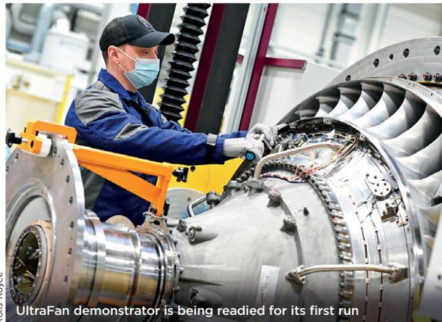
UltraFan demonstrator is being readied for its first run
