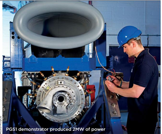
PGS1 demonstrator produced 2MW of power
