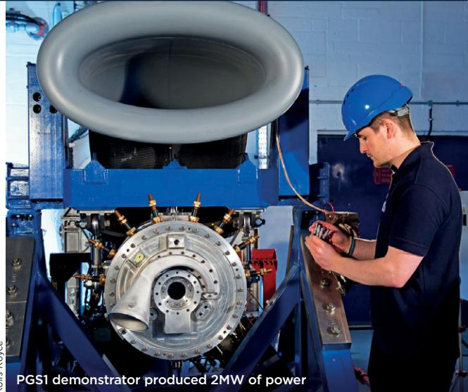
PGS1 demonstrator produced 2MW of power
