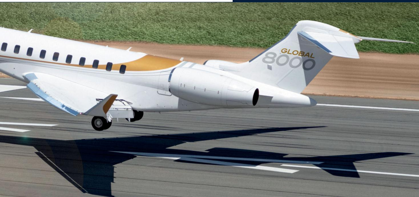
The Global 8000 will be 33.8m long, with 16.59m of useable cabin space, compared with respective figures of 30.4m and 14.27m for the G800.
